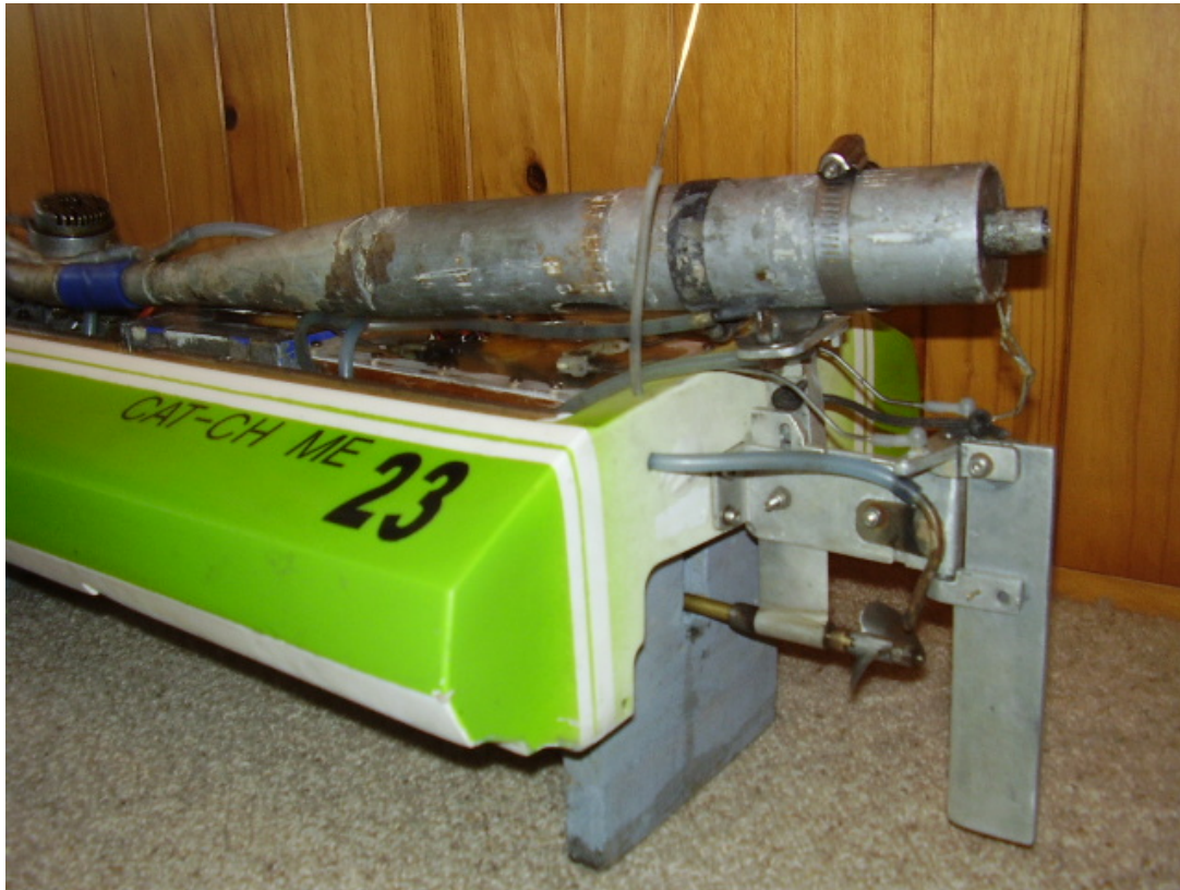
Figure 1: Connecting the pipe mount to the strut and an aluminium coupling under the silicone exhaust joint completed an electrical circuit around the radio box
