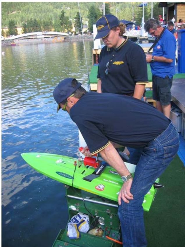
Fast starting a mono at Naviga 2006 – notice plug lead and belt through hatch!!
